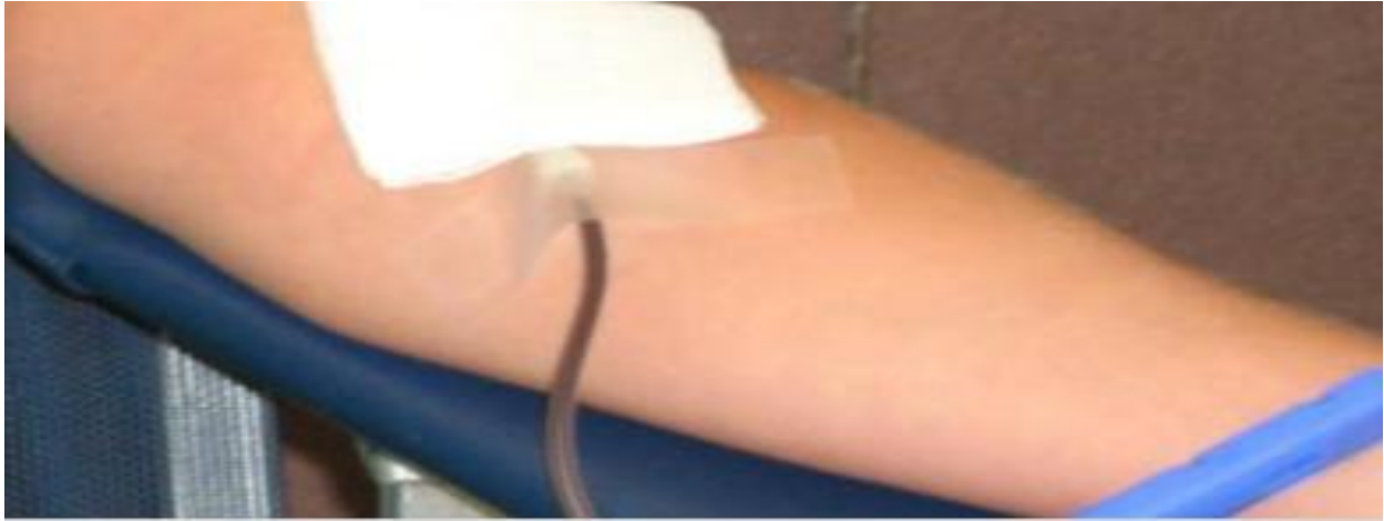
Fig. 3.3 LM 35 Sensor Which Measure the Body Temperature, the Sensor is Placed on the Hand
