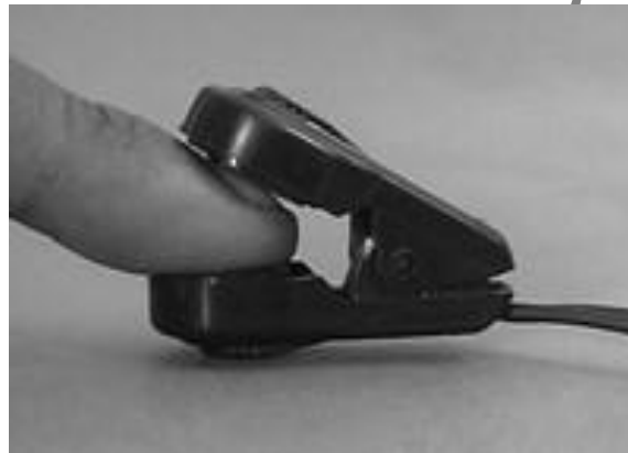
Fig. 2.5 Heartbeat Sensor Device
